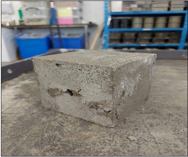
Figure 11. UHPFRC Cube After Failure
