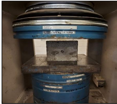
Figure 4. Cube Compression Test
