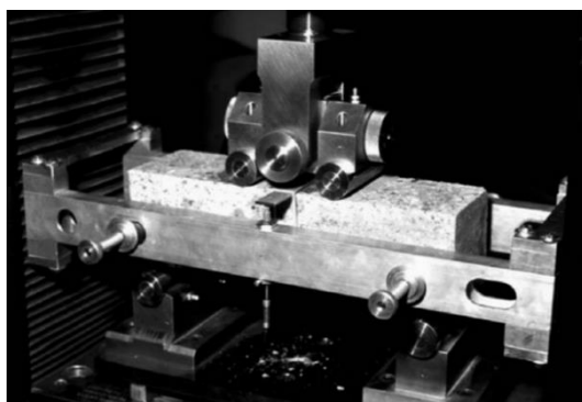
Figure 6. Rectangular Jig Surrounding the Specimen with Two Displacement Transducers Mounted at Mid-Span (ASTM C1609)
