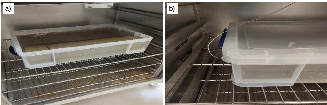
Figure 3. a) UHPFRC Specimens Placed in Oven for Heat Treatment; and b) Thermocouples Attached to The Boxes
