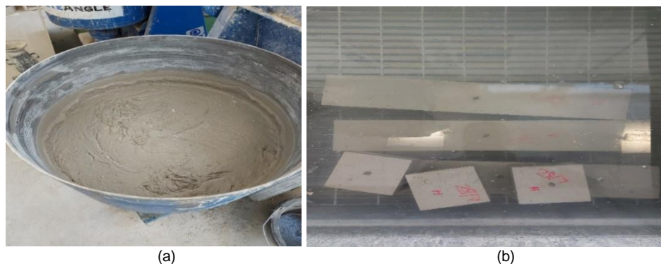
Figure 1. (a) Flowable UHPFRC Mix; (b) UHPFRC Specimens Water Cured at Room Temperature
