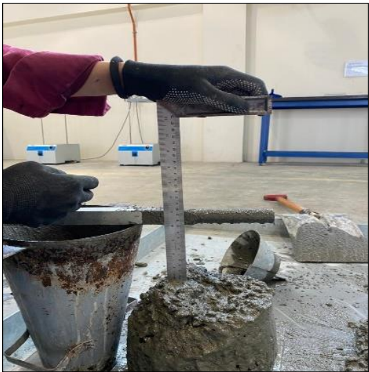
Figure 2. The Slump Test on Concrete Mix Design
