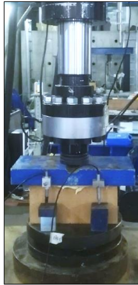
Figure 8. Setup Test for Determination of Deformation of Compressed Earth Blocks
