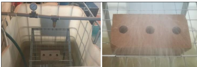
Figure 11. Rain Erosion Test Procedure
