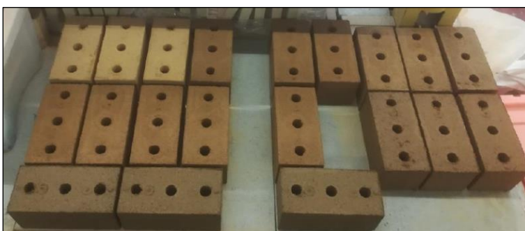
Figure 3. Produced Specimens with Dimensions of 220x105x135 mm 3
