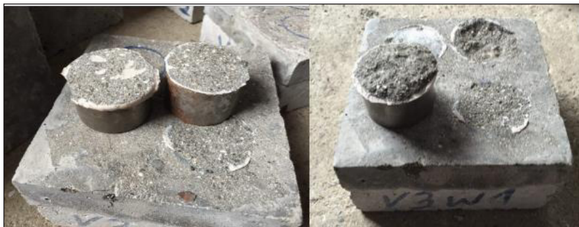
Figure 2. determination of in-situ strength of repair layer using Pull-Off (without coring)
