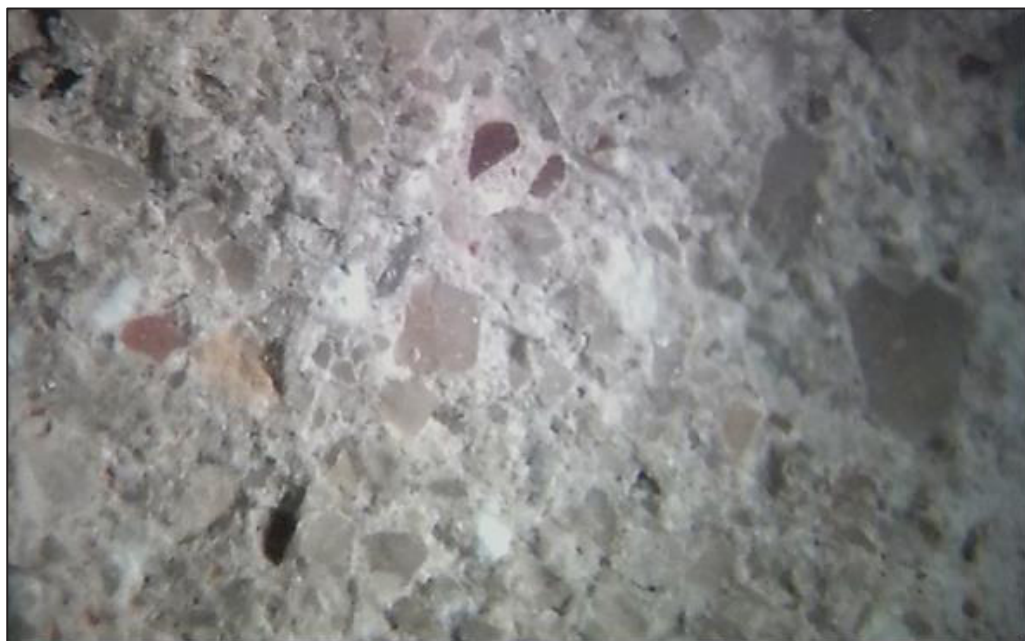
Figure 6. Macrostructure of carbonized test samples of calcareous and limestone compositions based on marbleized limestone, \times 100
