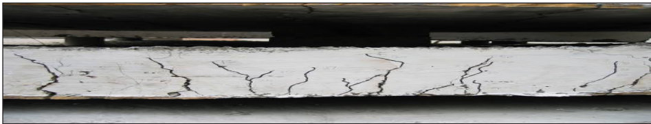
Figure 5. Photograph showing the propagation of cracks in the semi precast OPS slabs
