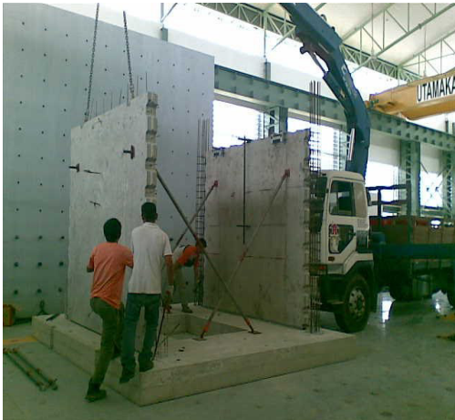
Figure 2. Precast shear-key wall is placed on pad footing at strong floor.
