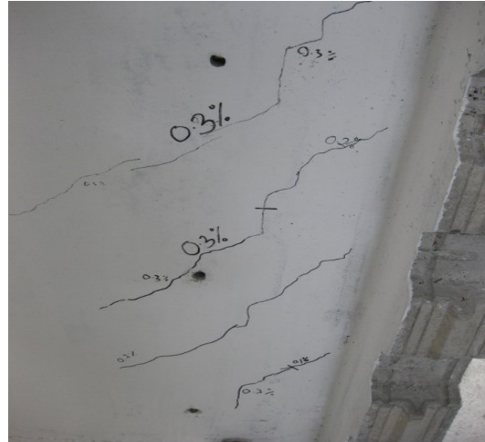
Figure 9. More hairlines cracks were observed at +0.3% drift with cracks width of 0.5mm.
