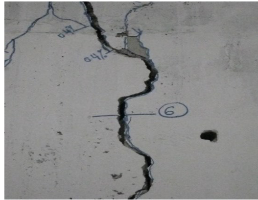
Figure 13. Cracks on wall-column interface during 0.7% drift at Point 6
