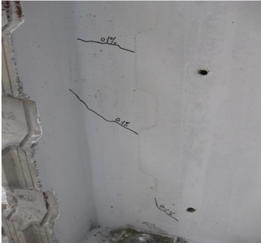
Figure 8. Hairline cracks observed at +0.1% drift between the joint of wall and column.
