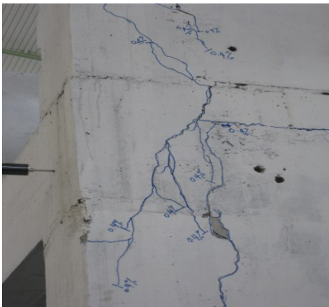
Figure 10. Cracks occur at first floor beam during +0.4% drift.
