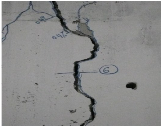
Figure 12. Cracks on wall-column interface during 0.6% drift at Point 6.
