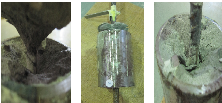
Figure 10. Bar Slippage from Left to Right: P15 D55, P25 D55 and P35 D55
