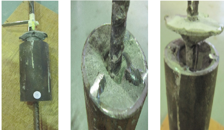
Figure 8. Bar Slippage from Left to Right: P15 D35, P25 D35 and P35 D35
