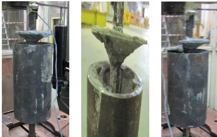
Figure 9. Bar Slippage from Left to Right: P15 D45, P25 D45 and P35 D45
