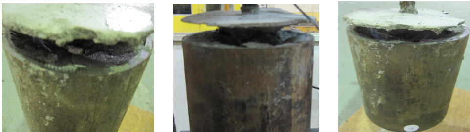
Figure 13. Bar Slippage from Left to Right: P15 D85, P25 D85 and P35 D85
