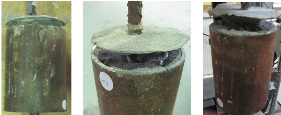
Figure 12. Bar Slippage from Left to Right: P15 D75, P25 D75 and P35 D75
