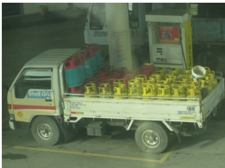
Figure 1. A truck arrived at PFS contains numbers of gas cylinders. It can be a potential source of ignition and cause of high scale fire event.
