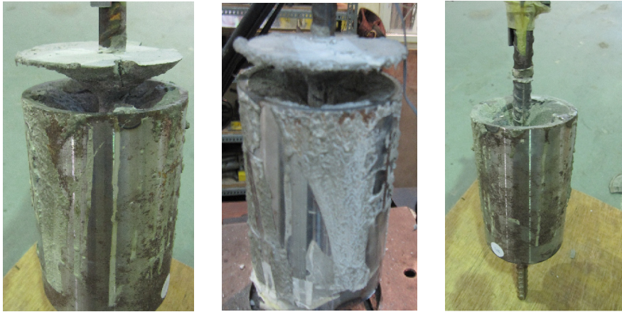
Figure 11. Bar Slippage from Left to Right: P15 D65, P25 D65 and P35 D65
