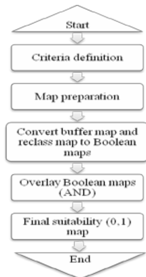
Figure 2. Procedure of Boolean Intersection
