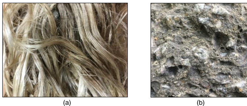
Figure 1. (a) KenafFibre and (b) Kenaf Fibre with Concrete
