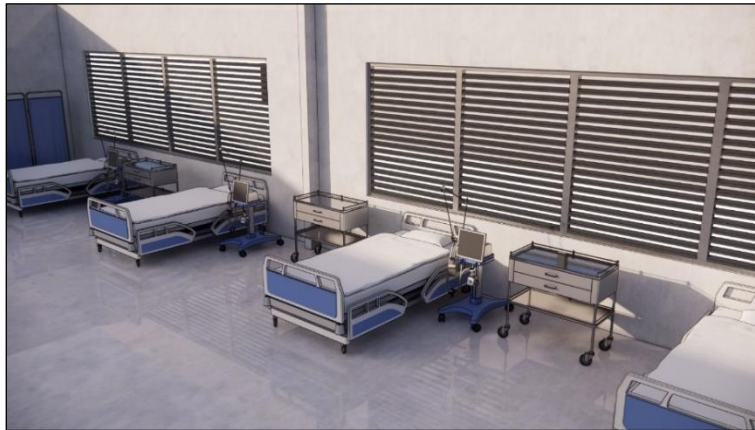
Figure 3. Mounted Louvers are Proposed to Effectively Block Excessive Glare
