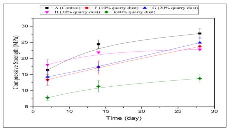
Figure 8. Compressive strength of various percentages of quarry dust with 0% (control), 10%, 20%, 30% and 40% at different ages (7, 14 and 28 days)
