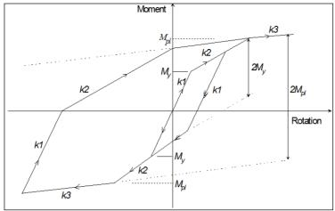
Figure 3. Analytical connection model response to a general load history
