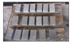
Figure 3. Air curing
