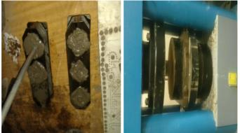
Figure 3. Preparation of mortar cubes and the compression test equipment Results and analysis for GP cement mortars
