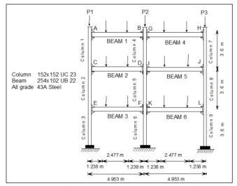
Figure 16. General arrangement of the frames SUF2
