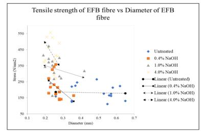
Figure 8. Tensile strength of EFB fibre againts diameter for untreated and treated fibre
