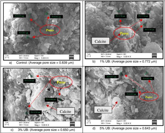
Figure 4. Pore measurement for control and bacterial ICEB
