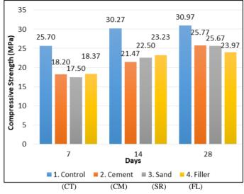
Figure 7. Compressive Strength of Cement Mortar against Time
