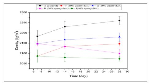
Figure 6. Density of different percentages of quarry dust with 0% (control), 10%, 20%, 30% and 40% at various ages (7, 14 and 28 days)
