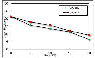
Figure 7. Variation of linear shrinkage of landfill soil with OPC and BA content
