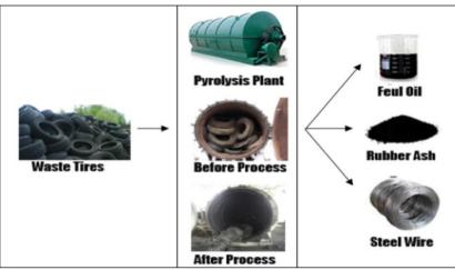
Figure 1. Pyrolysis process
