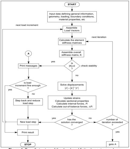
Figure 4. Overall structure of the developed finite element procedures
