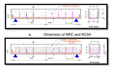
b. Dimension of RCAI Figure 2. Dimension of NRC, RC9A, and RCAI beams
