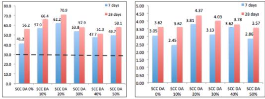
Figure 6. Compressive strength and tensile strength for SCC DA%
