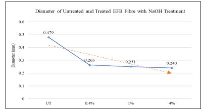
Figure 6. Diameter (mm) of Untreated Fibre (UT) and fibre treated with 0.4%, 1% and 4% concentration of NaOH
