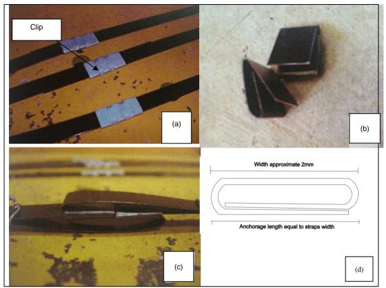
Figure 4. Connection: (a) conventional clip for box packaging; (b) new clip; (c) elevated view of the connection; (d) schematic diagram of the clip connection
