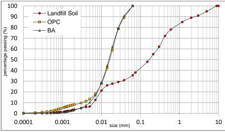
Figure 2. Particle Size distribution for Soil, Cement and Bagasse Ash
