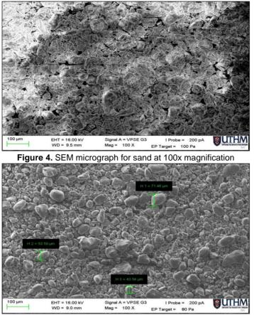
Figure 5. SEM micrograph for rubber ash at 100x magnification
