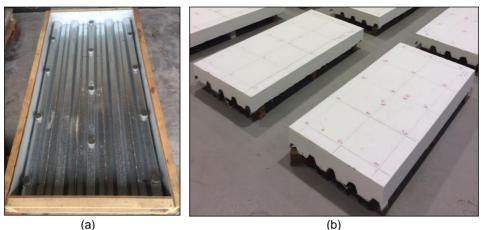
Figure 4. Specimen preparation of composite slab: (a) Mould and (b) Hardened composite slab
