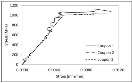
Figure 3. Measured stress-strain curves of steel straps (Ma et al., 2014a)
