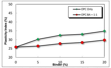
Figure 6. Variation of plasticity index of landfill soil with OPC and BA content
