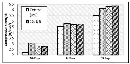
Figure 1. Compressive strength of control and bacterial ICEB
