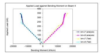
Figure 13. Total Applied Load against Bending Moment on Beam 4
