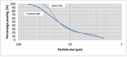
Figure 3. Comparison of particle distribution between raw CBA and treated CBA
