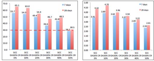
Figure 7. Compressive strength and tensile strength for SCC DA30% CR%
