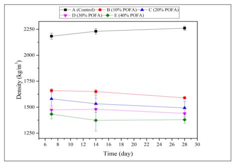
Figure 5. Density of different percentages of POFA with 0% (control), 10%, 20%, 30% and 40% at different ages (7, 14 and 28 days)
