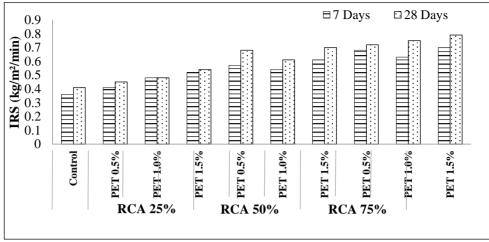
Figure 11. The average initial rate of suction of sand cement composite brick
