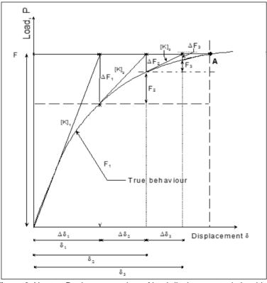
Figure 2. Newton-Raphson procedure of load-displacement relationships
