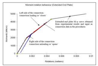
Figure 9. Loading-unloading connection behaviour at the top of the centre column of Figure 19 and 17
