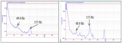
Figure 8. Natural frequency of beam before and after strike of 45 kA of electric current
