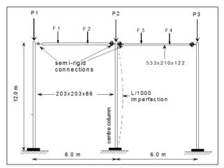
Figure 5. Frame used to examine the effect of loading and unloading behaviour of the connection
