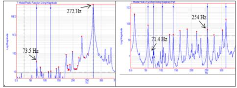
Figure 7. Natural frequency of beam before and after strike of 30 kA of electric current
