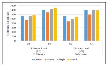
Figure 12. Effects of single and hybrid layer of FRP wrapped on ultimate load
