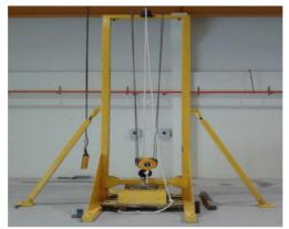
Figure 3. Drop weight Impact test equipment
