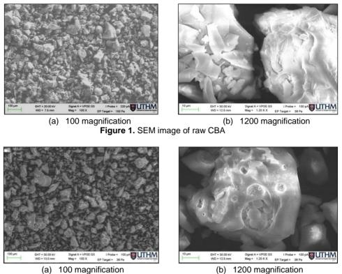
(a) 100 magnification (b) 1200 magn Figure 2. SEM image of treated CBA
