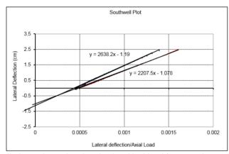
Figure 8. Southwell plot to determine the elastic critical load from results on the frame shown in Figure 6.
