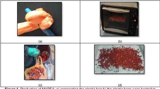
Figure 1. Production of MAPEA: a) compacting the plastic bag b) the plastic bags were heated to form the Artificial Polyethylene Aggregate (APEA) c) APEA encapsulated by glass and paint to produce MAPEA d) MAPEA ready to use as coarse aggregate
