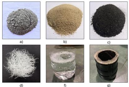
Figure 2. Main materials in foamed concrete; a) OPC, b) Sand, c) RHA, d) PMM), f) Foam agent and g) SP
