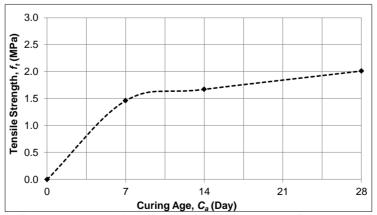
Figure 10. Tensile strength of foamed concrete containing 40%RHA and 9kg/m<sup>3</sup> PMM
