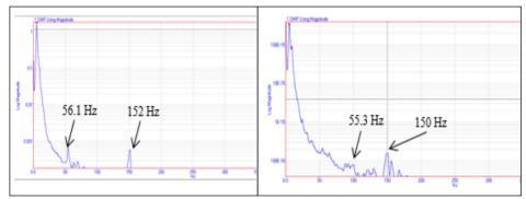
Figure 6. Natural frequency of beam before and after strike of 15 kA of electric current
