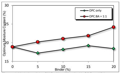
Figure 8. Variation of the OMC of landfill soil with OPC and BA content
