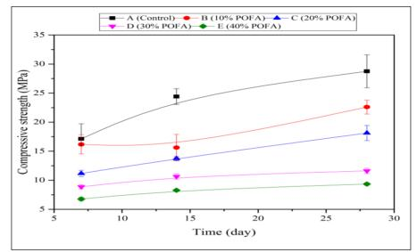
**Figure 7.** Compressive strength of different percentages of palm oil fuel ash with 0% (control), 10%, 20%, 30% and 40% at various ages (7, 14 and 28 days)
