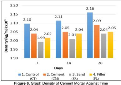
Figure 6. Graph Density of Cement Montal Against
