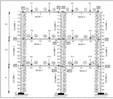
Figure 10. Modelling the BRE test frame for the analysis
