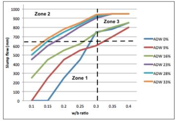
Figure 5. Effect of w/b ratio on slump flow in paste study
