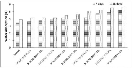
Figure 10. The average water absorption of sand cement composite bricks with RCA and PET
