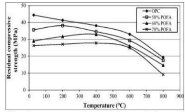
Figure 2. Effect of temperature on residual compressive strength of concrete (Awal and Shehu, 2015)
