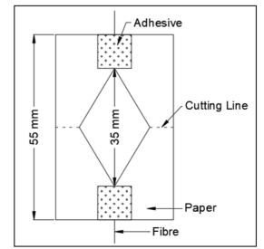
Figure 2. Schematic sketch of the experimental setup for tensile test
