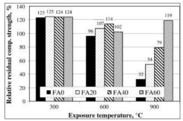
Figure 1. Relative residual compressive strength (Aydin and Baradan, 2007)
