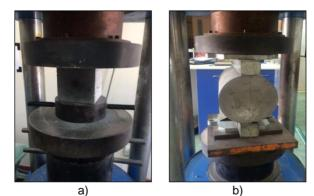
Figure 5. Test programme on cube and cylinder specimens, a) Compression test and b) Splitting-tensile test
