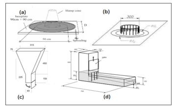
Figure 4. Fresh properties test (a) slump flow, (b) J Ring (c) V Funnel and (d) L Box
