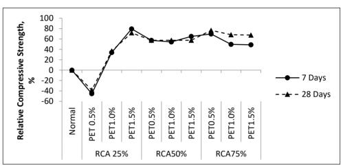
Figure 9. Relative percentage of compressive strength compared to normal brick
