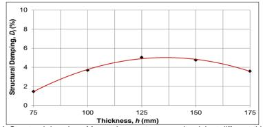
Figure 14. Structural damping of foamed concrete composite slab at different thicknesses
