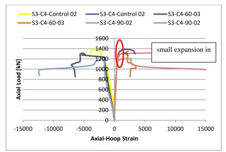
Figure 16. Axial load versus axial-hoop strain curves of Series 3 with to = 4 mm
