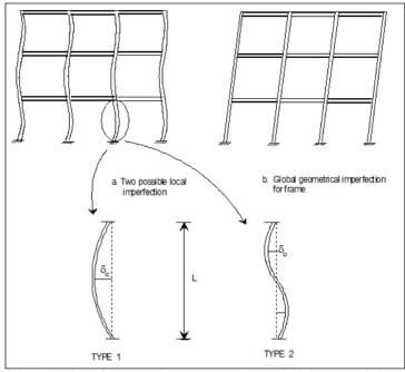
Figure 1. Modification of the input data to cater for the initial geometric imperfection
