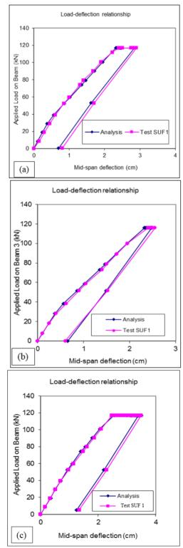
Figure 17. Comparison of the beam load-deflection response for SUF 1 at (a) Beam 2 (b) Beam 3 and (c) Beam 4
