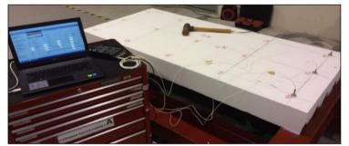
Figure 7. Test set-up for hammer-impact test
