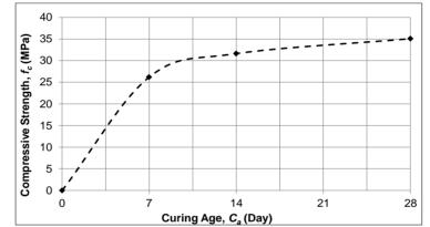
Figure 9. Compressive strength of foamed concrete containing 40% RHA and 9kg/m<sup>3</sup> PMM
