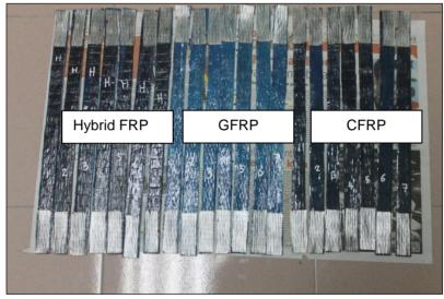
Figure 8. Witness panel for Hybrid FRP, GFRP and CFRP
