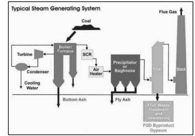
other remaining combustion products go out along the flue gas chimney. Figure 1 shows the combustion of coal to generate bottom ash in a thermal power plant.
