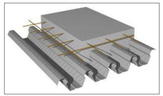
Figure 1. Composite slab consists of corrugated steel deck and reinforced concrete
