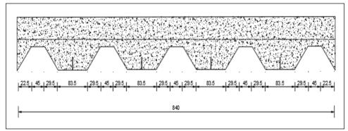
Figure 3. Schematic design of composite slab
