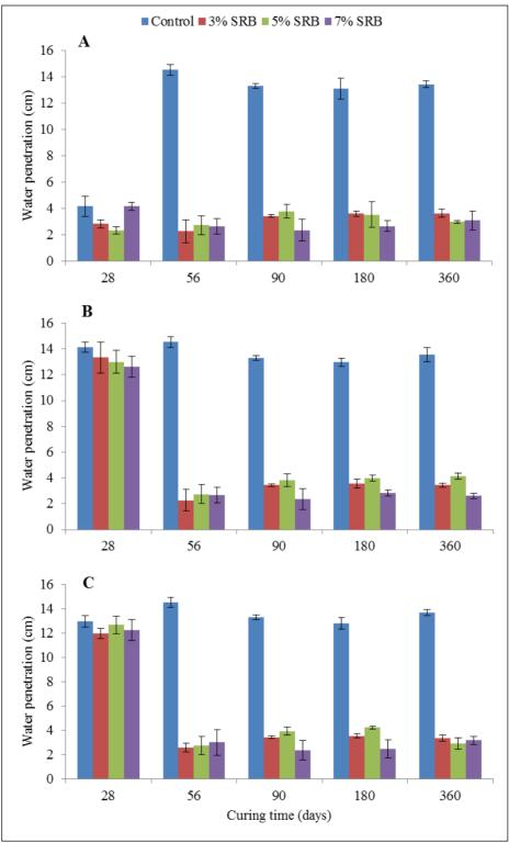
Figure 2. Water penetration with different percentage of SRB. A) 0.4 W/C ratio, B) 0.5 W/C ratio and C) 0.6 W/C ratio
