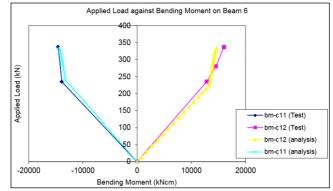
Figure 14. Total Applied Load against Bending Moment on Beam 6
