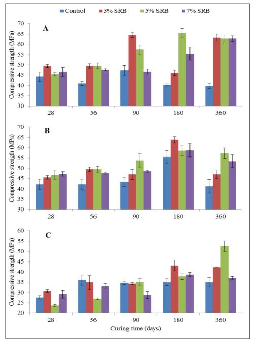
Figure 1. Compressive strength with different percentage of SRB as influenced by A) 0.4 W/C ratio, B) 0.5 W/C ratio and C) 0.6 W/C ratio
