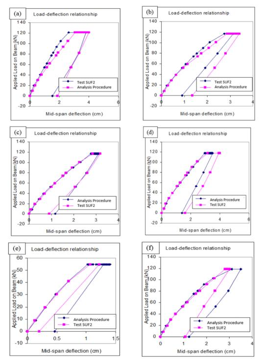
Figure 18. Comparison of the beam load-deflection response for SUF 2 of (a) Beam 1 (b) Beam 2 (c) Beam 3 (d) Beam 4 (e) Beam 5 (f) Beam 6
