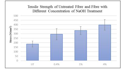
Figure 7. Tensile strength of Untreated Fibre (UT) and fibre treated with 0.4%, 1% and 4% concentration of NaOH
