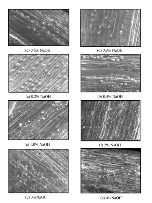
Figure 4. Scanning Electron Microscope (SEM) image at 250 magnification of Oil Palm Empty Fruit Bunch (OPEFB) treated with Sodium Hydroxide (NaOH) range 0.2% to 4% concentration
