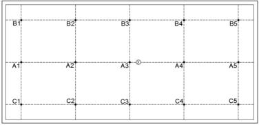
Figure 8. The position of the accelerometers during the test
