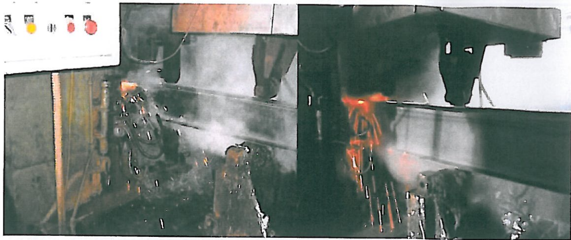
Figure 6 : Three steel strips welded by our high frequency welding process
