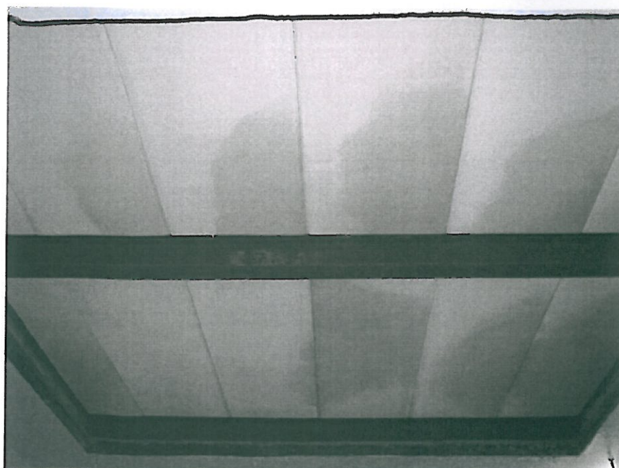
Figure 3 : Test setup of floor panel system installed on top of the reverberation room
