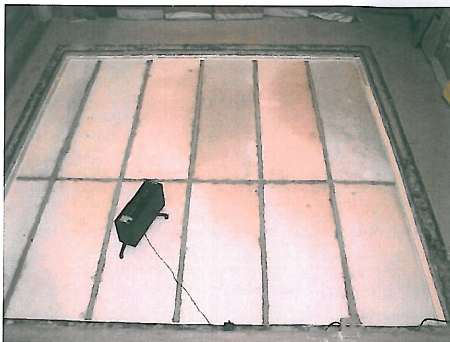
Figure 2 : Test setup of impact machine on floor panel system
